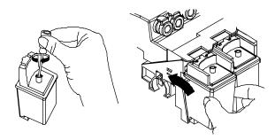
Install it bottom first into the correct slot on the carrier. DO NOT REMOVE THE BLUE
